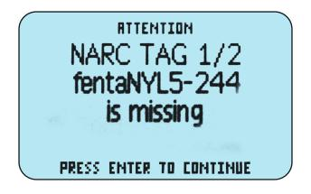
Press **ENTER** to continue to begin telling the NARC iD system the whereabouts of the missing controlled substances. Depending how the system has been configured in LockView there will be many choices available. These include **INCIDENT** or **CONSUMED**, **EXPIRED**, **LOST**, **BROKEN**, **SKIP** or **TRANSFER**. Press the **UP**, **DOWN** buttons or enter the number corresponding to the whereabouts directly.
