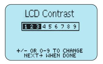
Use the +,- buttons to choose the contrast of the LCD display. Alternately, choose **1-9** directly to choose the contrast level. Press **NEXT** when done.
