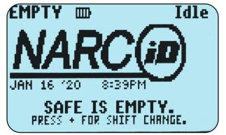
Type a valid PIN code or present a valid card to the credential reader to access the NARC iD box. (See CompX LockView software instruction manual for information regarding adding valid users.) Open the door and insert a tote containing RFID enabled capsules with tags. When the door is closed, the NARC iD system will turn on and scan the box for tags. The LCD screen will say **SCANNING DRUGS PLEASE WAIT**. It will also show how many tags have been identified / confirmed.
