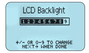
Use the +, - buttons to choose the brightness of the LCD display. Alternately, choose **1-9** directly to choose the brightness level. Press **NEXT** when done.
