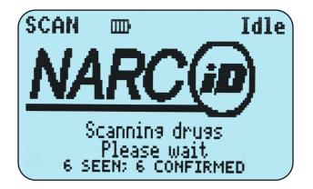
After the NARC iD system has completed the scan, the LCD will show how many tags are in the safe
