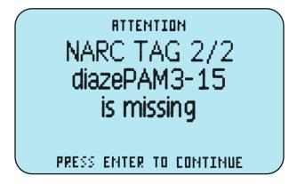
If the location of a specific missing tag is unknown or you desire to enter the information later, you can choose **SKIP**. If this is chosen, the NARC iD system will continue to ask about this missing tag after each scan.
