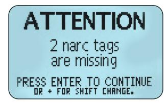
Press **ENTER** to continue. You will be asked about each missing tag. If multiple tags are missing, you will see which tag is being asked about along with the total inquiry. In this example, the LCD says **NARC TAG 1/2 fentaNYL 5-244 is missing**.
