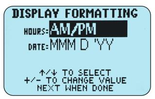
Choose the hour format (AM/PM or 24 hour) by using the **UP** and **DOWN** keys to highlight the words to the immediate right of HOURS. Use the + and – buttons to change the selection.
