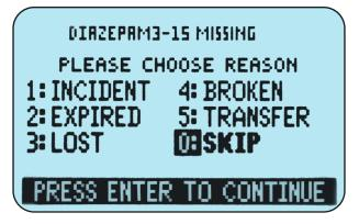
After the whereabouts of each missing tag have been entered the LCD will show the current contents of the box. If **SKIP** was chosen for any tags, the LCD will show how many tags are still unaccounted for.
