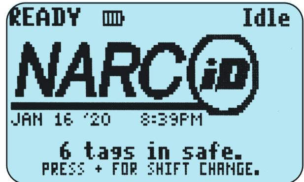
Access the NARC iD CSU system with a valid credential and remove the tote (along with ALL tags). Close the door. The NARC iD CSU system will scan the contents of the CSU and the LCD will say **SAFE EMPTY XX TAGS MISSING**. (If all of the tags were not removed, you will be immediately asked about the reason the tag is missing, see below).
