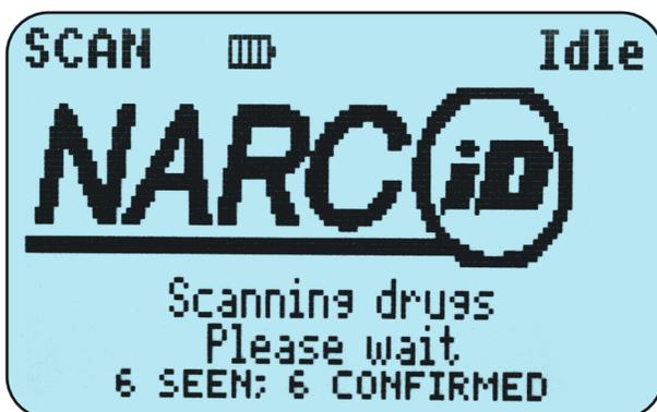
After the NARC iD CSU system has completed the scan, the LCD will show how many tags are in the safe.
