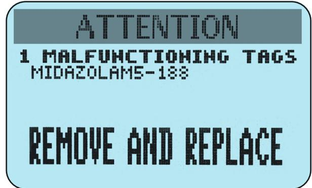
When this happens, remove the controlled substances that are noted on the screen. Review **NARC-iD Capsule Assembly Instructions** (page 9). Verify that the locking tab is fully inserted as noted in **step 5**. After this has been verified, try using the capsule again. If the tag continues to malfunction, try a new cap/tag.
