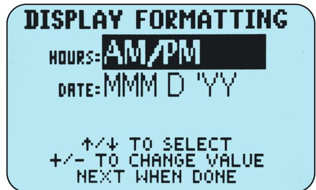
Choose the hour format (AM/PM or 24 hour) by using the **UP** and **DOWN** keys to highlight the words to the immediate right of HOURS. Use the + and - buttons to change the selection.
