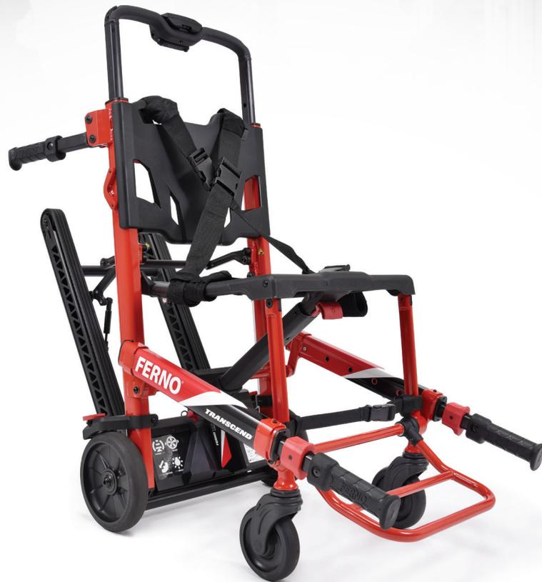
The **Transcend™ Stair Chair with PowerTraxx®** provides maximum safety and power when transporting a patient up or down stairs. Its electronically-controlled motor, direct drive transmission, and powered tracks push and pull patient loads of up to 550 pounds. The chair and track system carry the weight, increasing patient safety and reducing operator fatigue and risk of injury.
