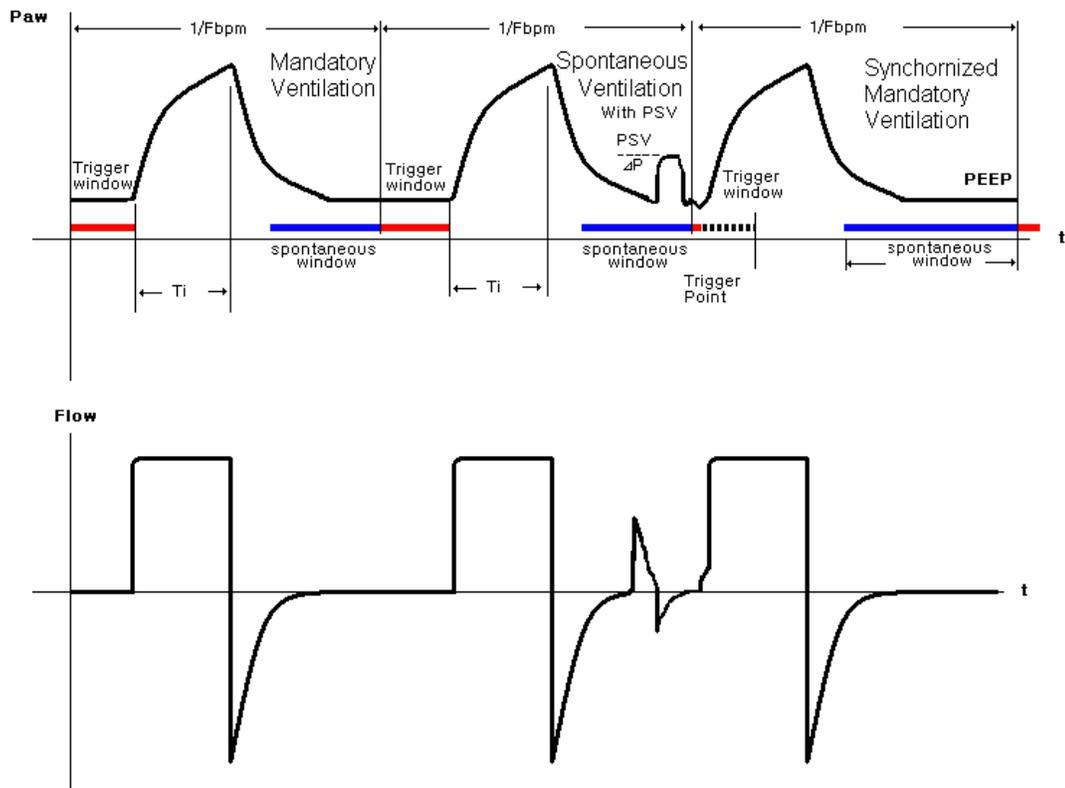
Figure-11.b SIMV waveform with pressure support
