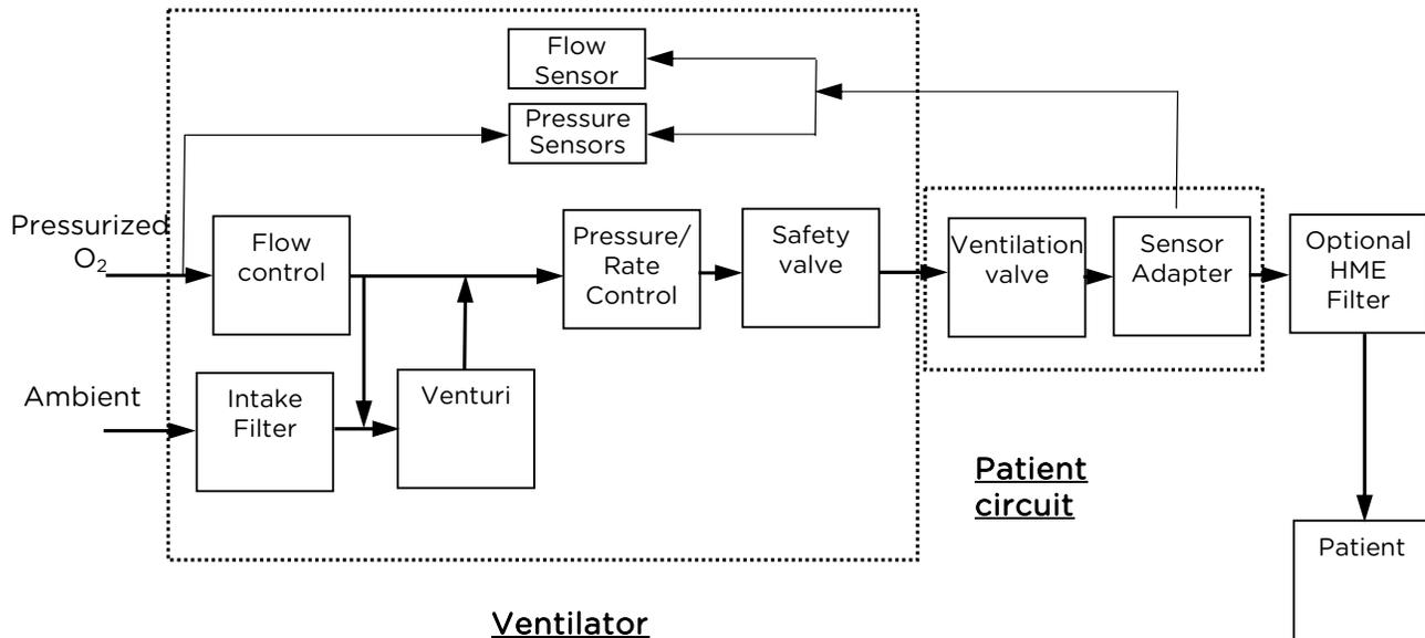
When a gas source (medical oxygen) is supplied to the e700 ventilator via the gas input connection, the gas will flow into the Flow control valve which is used to control both the flow and rate of ventilation. The output of this valve is connected to a selector switch which is used to direct the flow path either directly to the ventilator output (if 100% oxygen ventilation is required) or through a Venturi system used to entrain air to provide an oxygen concentration of 60%.
